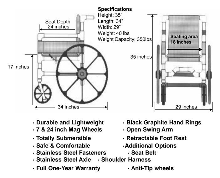
All **AQUATREK** aquatic wheelchair models are designed for use in and around water. Its unique design allows full usage in swimming pools, spas, splash pads, leisure rivers and showers. Its construction from PVC plastic and stainless steel fasteners makes it both durable and non-corrosive.
